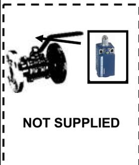
Position switch may be connected to the emergency circuit.
